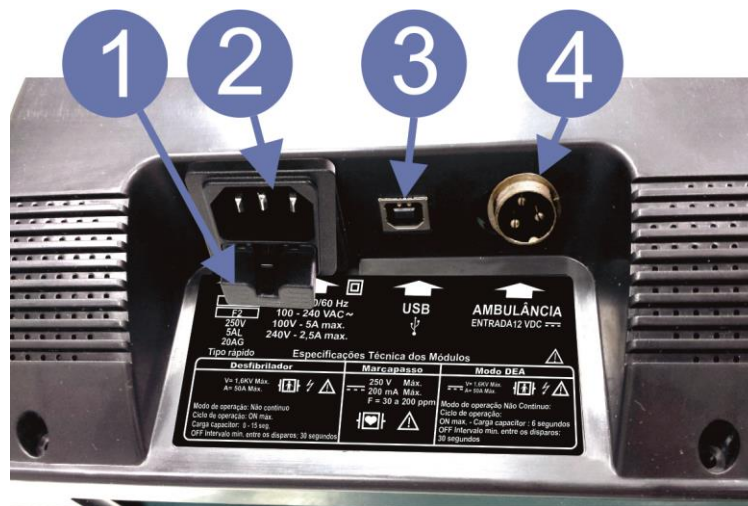
Figure 5 – Power and communication inputs.
